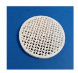
This ready-to-use alumina paste has been developed for Robocasting 3D printing.
